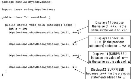
Figure 6-4: Preincrement and postincrement. }
